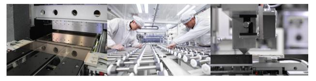
Manz@work in display manufacturing: The Manz G2 Slit Coater for photoresist coating in the touch panel litho production. Manz G2 Slit coater eliminates substrate damages as caused by conventional transmission approaches. Equipment for touch panel manufacturing at Manz in Asia.
