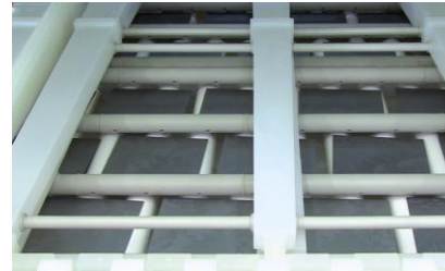
Chemical Edge Isolation process: Single side etching process which etches away the PSG- and the highly doped layer from the backside of the wafer.
